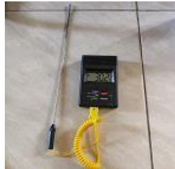
Gambar 4. Termometer Digital TM-902C
