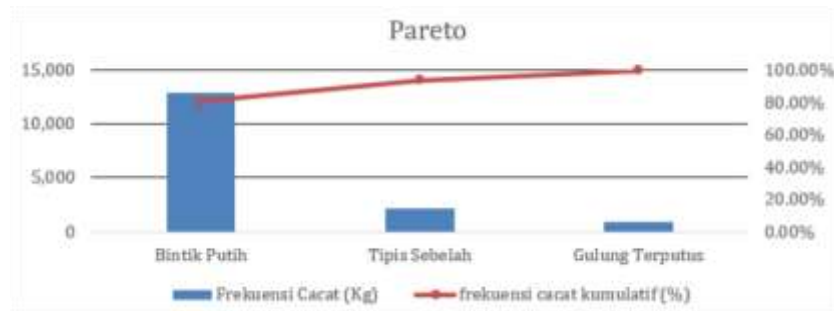
Figure 2. Pareto Diagram of the Number of Types of Defects in Plastic Bags Size 24
